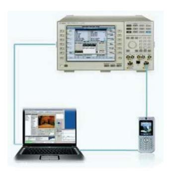
Figure 1: Test mode BER and MS calculated BER without a signaling connection or TCH loopback will reduce Rx test times
